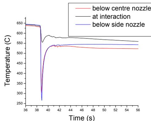
Figure: a. Three water jets impinging on moving hot steel plate;b. Cooling curves below nozzles and at interaction, for Flow rate = 30l/min, with two jets 3 inches apart and plate speed = 0.22m/s
