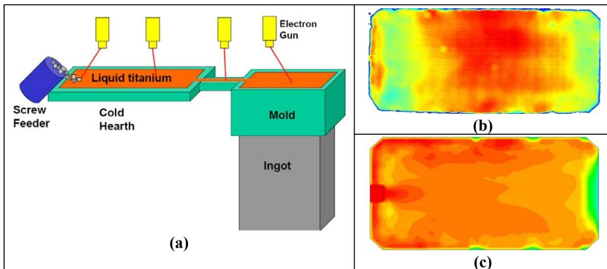
Figure 1: Schematic illustration of electron beam cold hearth melting (a), and temperature contours on ingot top surface from experiment (b) and model (c)
