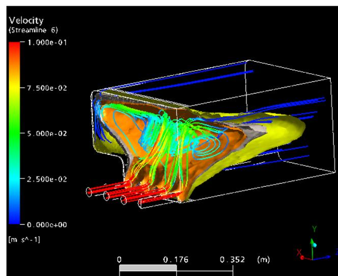
Predicted solidus (yellow), 30% fs (grey), liquidus (orange) surfaces are shown with streams (coloured based on velocity) for T-ingot casting of A356 in the z-direction
