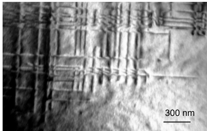
Plan-view TEM micrograph of misfit dislocations lying along  $\langle 110 \rangle$  directions in an InGaNA film grown on an (001) single crystal GaAs substrate
