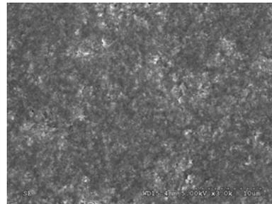
Figure - Surface of dried pastes with a same P(powder)/L(liquid) ratio but different amount of EG and TSC . A left SEM micrograph of the dried paste A shows highly agglomerated lump of HAP causing bad flowability and high viscosity compared to smooth surface of the dried paste B.
