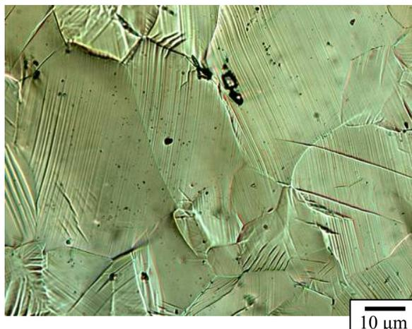
*Slip markings in AZ80 alloy deformed to 5 % strain at 77K*
