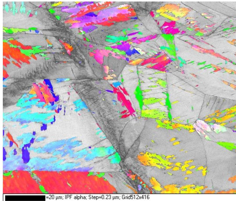
EBSD orientation map showing austenitic grains (in grey) filled with martensite variants (coloured).
