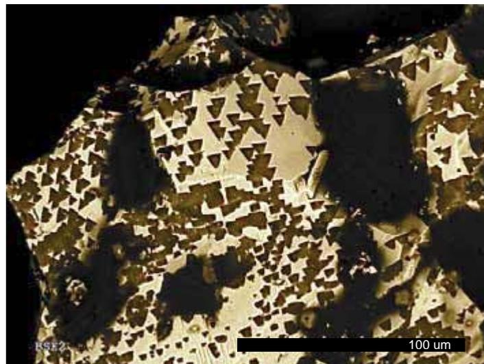
**Figure 1:** SEM Micrograph of a single chalcopyrite particle (1M H<sub>2</sub>SO<sub>4</sub> + 1M NaCl) at 30 seconds of transpassive leaching.
