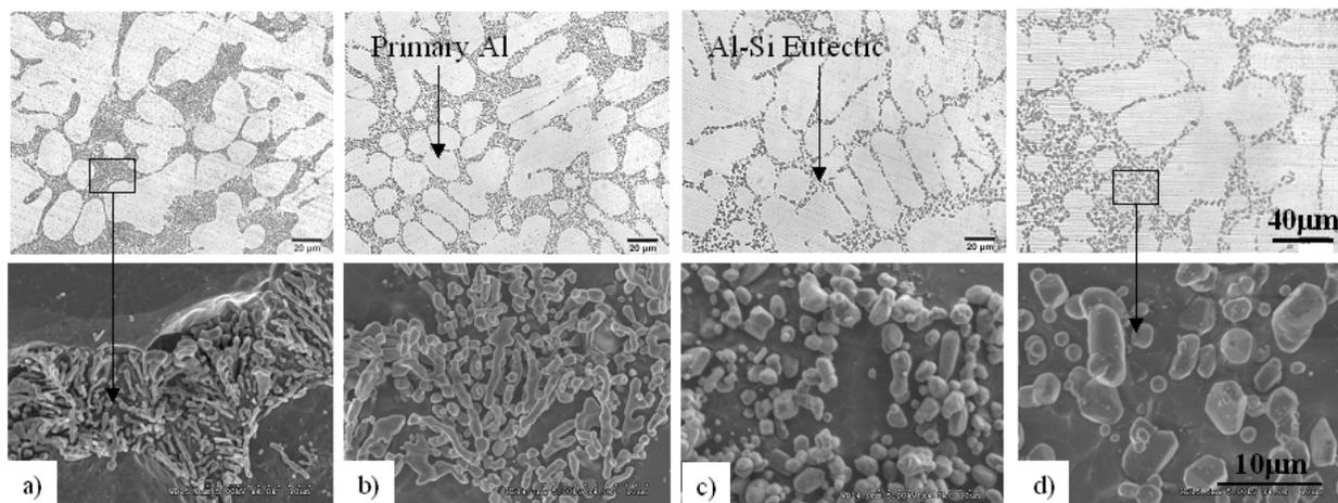
Optical (top) and deep etched (bottom) micrographs illustrating the modification of eutectic silicon particles in the A356 alloy during solution treatment;
